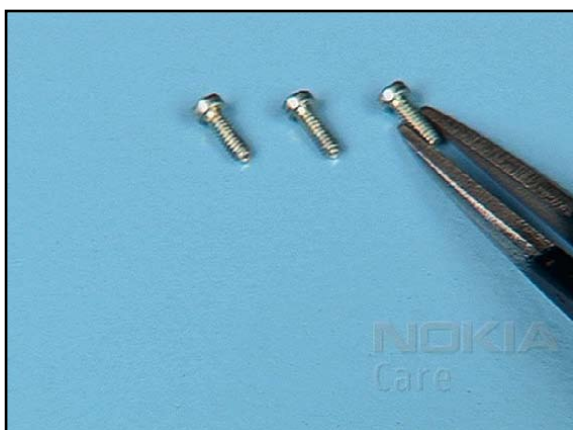
23. Use the medium lengths of the new screws.
