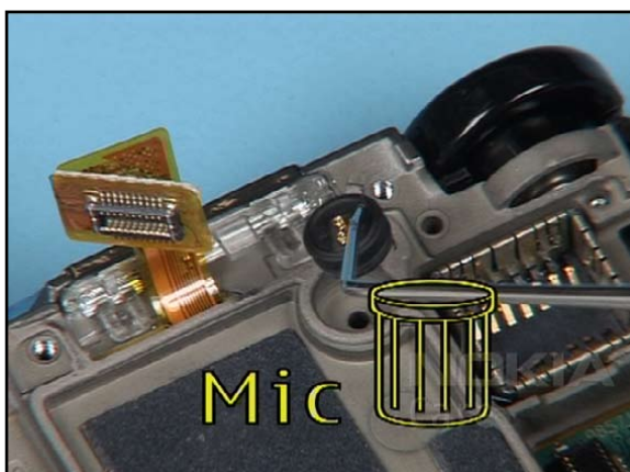
23. Remove the MICROPHONE and discard it.
