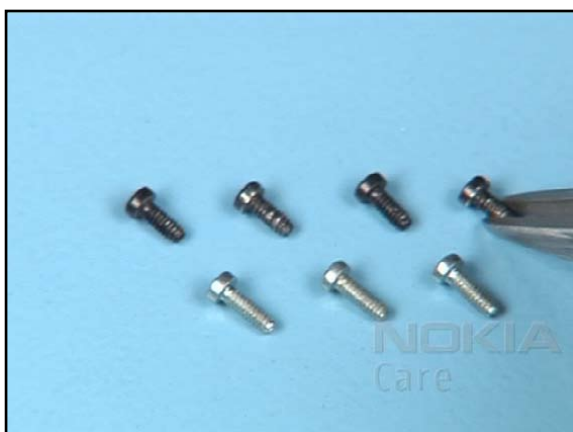
23. Use the black and shortest ones of the new screws.
