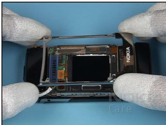
14. Place the B-COVER DECO as shown.
