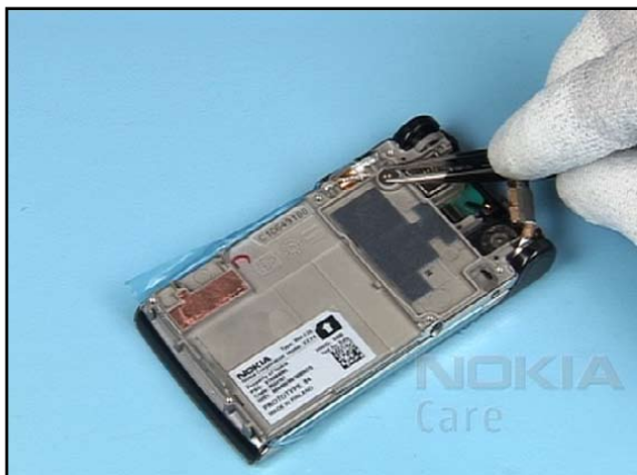
13. Insert the MICROPHONE.
