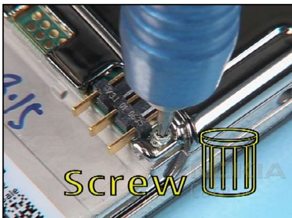
9. Unscrew this screw and discard it. Do not use it again.
