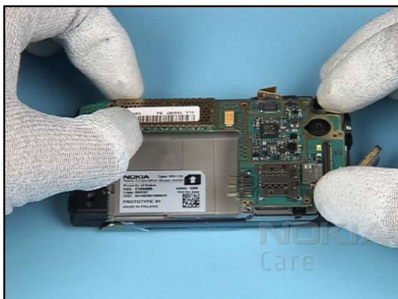
19. Bring the ENGINE MODULE into position as shown. Push it slightly into place vertically, ensure that the hidden connector is correctly positioned before continue.
