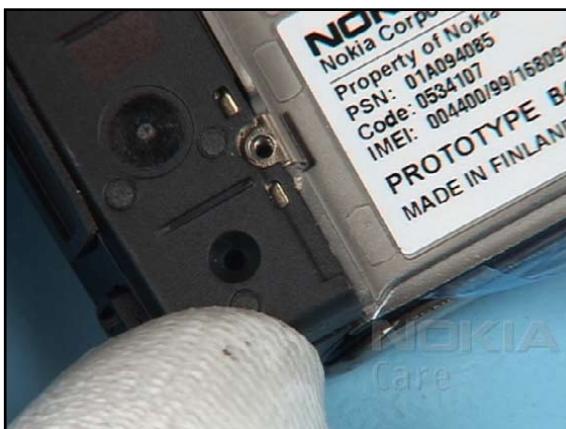
18. Place the ANTENNA MODULE. Mind the guides.
