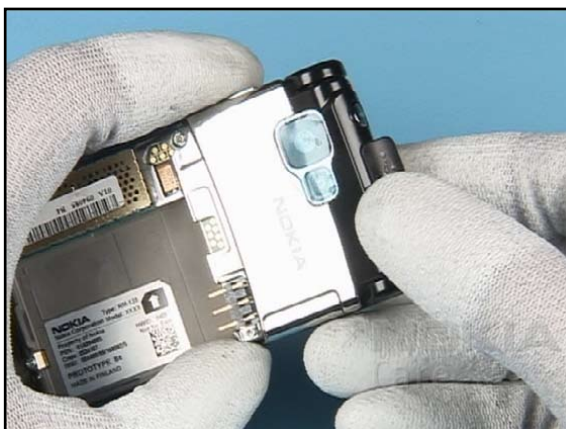
28. Align the HINGE COVER BOTTOM first. Slightly click the snaps into their places.
