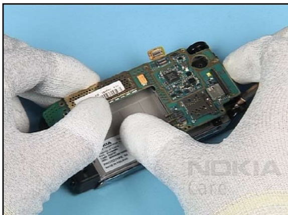
19. Lift up the ENGINE MODULE vertically. Note that this module is connected with a hidden connector.
