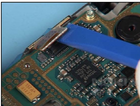
16. Open the flex foil connector.
