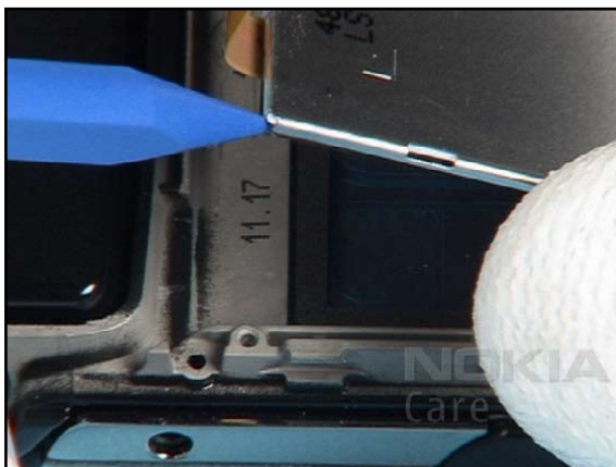
22. Carefully lift up the LCD and shift it into direction shown.
