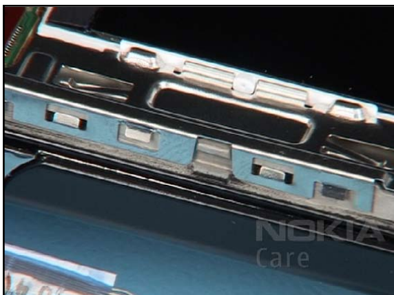
12. Note the correct positioning and click the snaps into their places.
