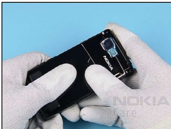
8. Another option for SD D00R removal is shown here. Remove the BATTERY COVER.
