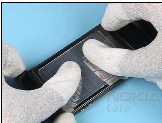
34. Smooth the KEYMAT into center position.
